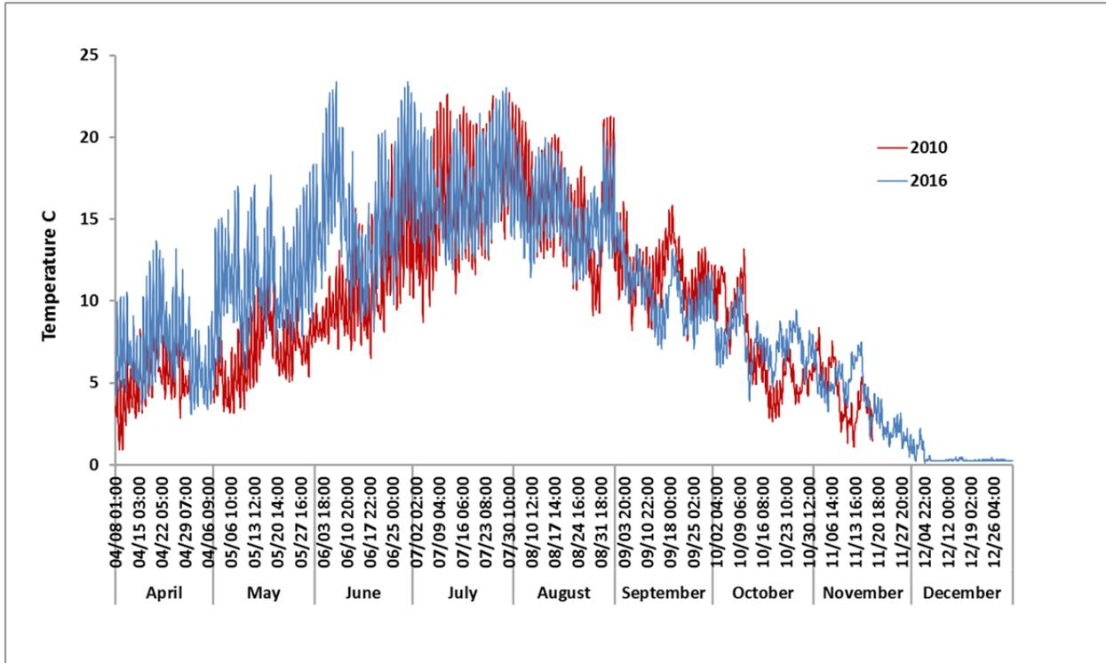
**FIGURE 30** PLOT OF THE DIURNAL FLUCTUATION IN WATER TEMPERATURE AT THE LOWER PROJECT SITE (RIVER MILE 0.06) FOR 2010 AND 2016. PLOT SHOWS THE REDUCTION IN DIURNAL FLUCTUATIONS OF WATER TEMPERATURE RECORDED AT THIS SITE IN 2016 COMPARED TO THE PRE-PROJECT/ DATA OF 2010.
